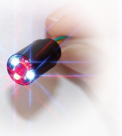
Optical DO sensor LED's flash during measurement.
